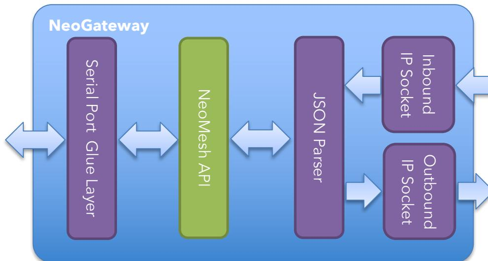
The architecture is such that payload data being send from a node inside the NeoMesh network to the gateway node, will be delivered on the Outbound IP Socket in JSON format. Similarly, payload data being send from the IP network shall be send as a JSON formatted package to the inbound IP Socket.
